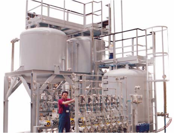
Glycol and Corrosion Inhibitor Injection Package
